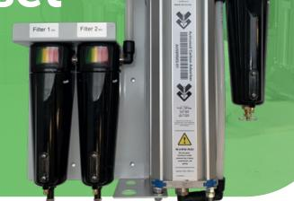
However, it is an excellent general filtration set-up for other applications as well. The set consists of two high efficiency coalescing filters to remove all particles and droplets. The carbon adsorber (bed type) removes all traces of compressed oil vapour (over a much longer period than traditional carbon filter elements) and ozon. A final dust filter prevents carbon dust carryover.
